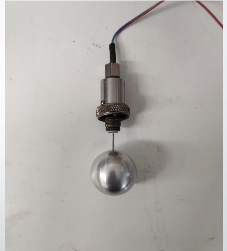
Figure 7. Aluminum sphere used, along with the thermocouple used for temperature monitoring.
