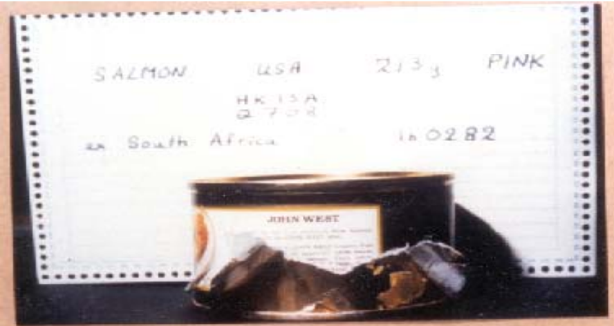
75 South Africa Can showing defect similar to the index can 76 Close up of 75
