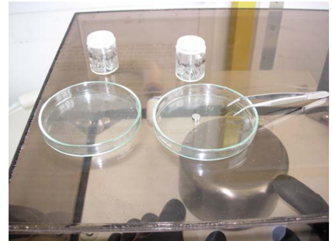
DSC-pans on top of the furnace
